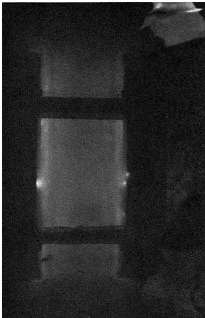
Fig. 2. Glow discharge obtained with a TFE flow rate of 1 \text{ cm}^3(\text{S.T.P.})/\text{min} , p_M = 300 \text{ mTorr} , and no magnets. Exposure time = \frac{1}{2} sec.
